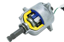
Mechanical Clutch Units for Next-generation Steering Systems (MCU)
